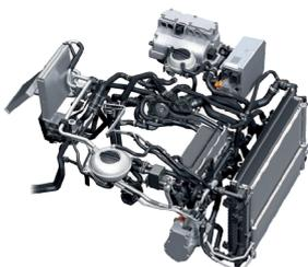
In the Audi A3 e-tron, for instance, the system conditions the cabin as well as cooling the internal combustion engine, gearbox and high-voltage components. All are integrated into the various cooling circuits, with the thermal management system controlling each element to ensure that they reach and maintain their individual optimum operating temperature as quickly as possible.
